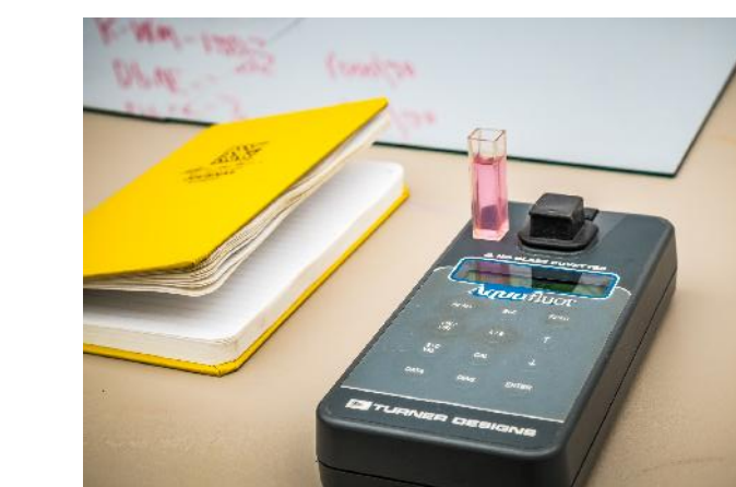
Tracer dye was mixed with the surfactant water mixture to further assess injection distribution.
