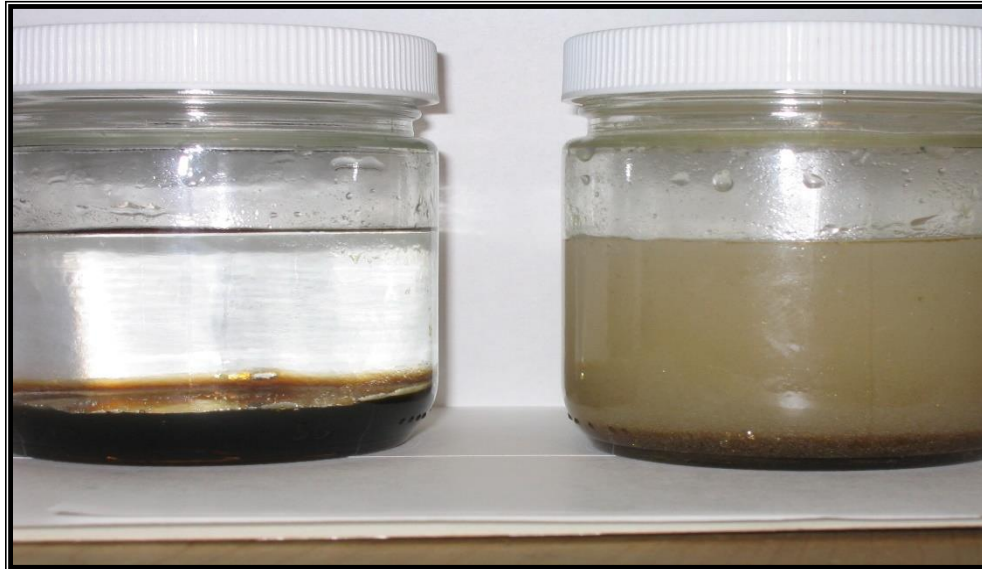
Photograph 2-3: Pre-post Ivey-sol ® DNAPL Remediation. Increasing the miscibility of the DNAPLs in the groundwater phase for enhanced extraction (i.e., PCE, TCE, CTC, PCB, etc.)
