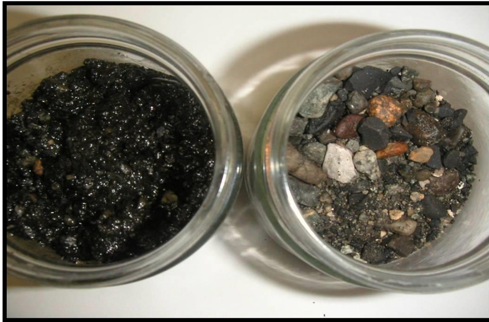
Photograph 2-1: Pre-post Ivey-sol® Remediation of Refinery Soils
